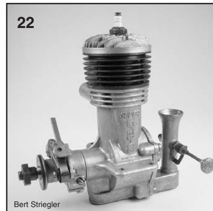
22 - SUPER CHAMPION - 1948 - .630 in 3 spark. Similar to Atwood "JH" Champion, but has "SUPER CHAMPION" on bypass. Small narrow bypass.
