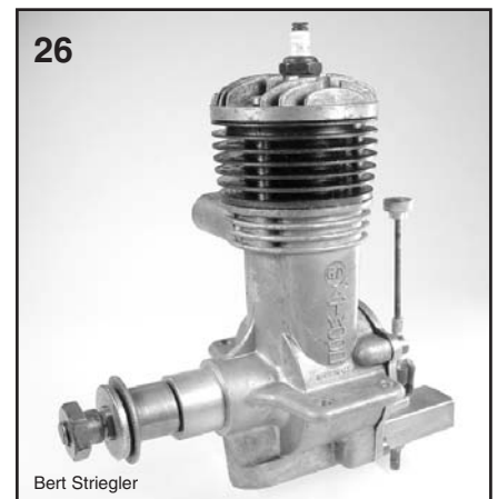
26 - GLO-DEVIL Model "GD" - 1948 - .625 in 3 glow. Like previous but without timer. "GD" on bypass.
