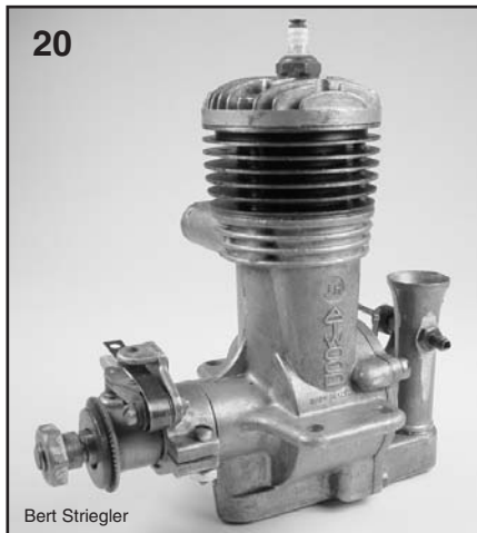
20 - ATWOOD SUPER CHAMPION (Model "JH") - 1946 - .611 in 3 . Lapped or ringed piston as #19. Exhaust now on opposite side from all previous models. "JH" in circle above vertical "ATWOOD" cast on bypass. Large bypass.
